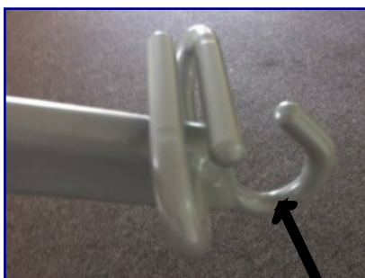
Hooks free from wear or damage
