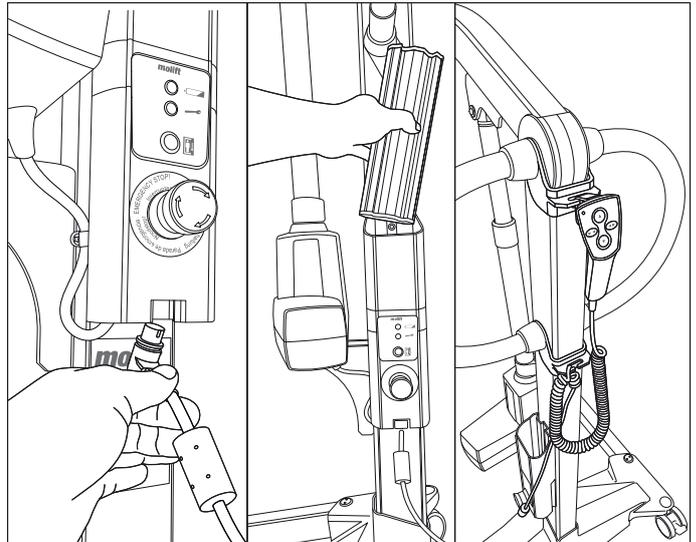
1. Connect hand control to bottom of battery holder.
