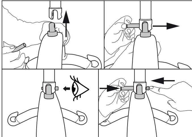
1. Align suspension in connection point.
