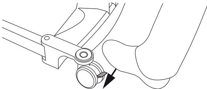
Rear wheels/casters are equipped with brakes. Step on lever to lock brakes. Flip up to unlock.
