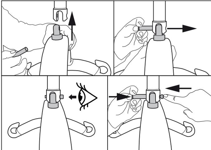
1. Align suspension in connection point.
