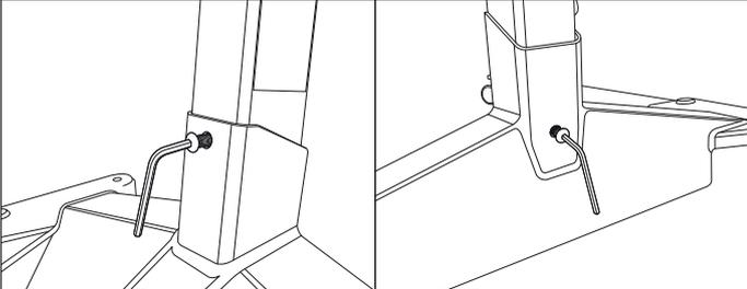
Lock the lift column in place by fastening the two hexagon socket screws in front and rear of the chassis.
