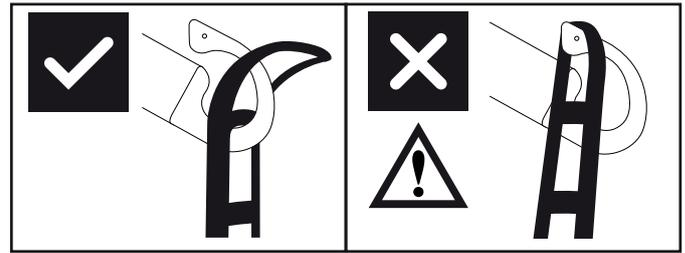
The suspensions hook design prevents sling to be inadvertently detached when mounted correct.
