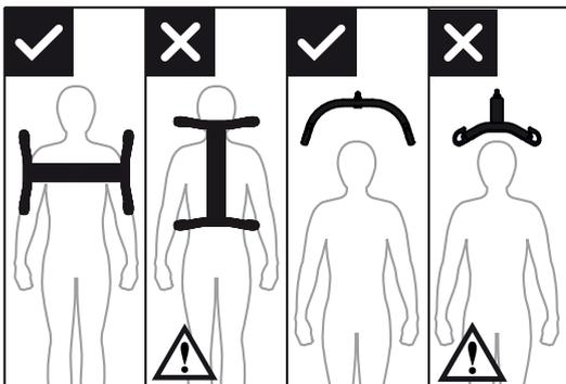
The 4-point suspension must always be positioned across the user, to prevent the user from unintentionally sliding out of the sling.
