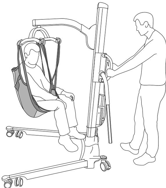
Try to position the user as low as possible (preferably resting the feet on the chassis) when transferring the lifter with a suspended user. In this way the centre of gravity will be low and reduce the risk of instability.
