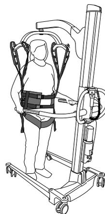
Lifter can be delivered with supporting arms, or complete lifting column with supporting arms can be delivered as an accessory to swap with original lifting column.
