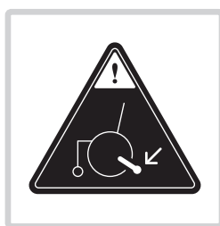
Risk of tipping: Always keep the anti-tips folded down.
