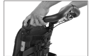
Fig. 52 Rotate Push Button downward
