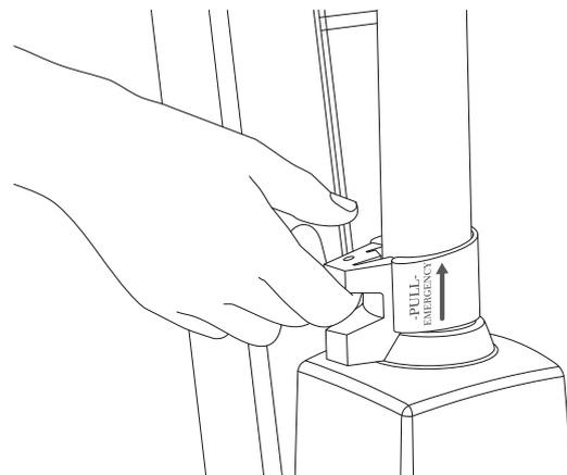
Pull handle on the actuator upwards to start emergency lowering, and the lifting arm moves downwards if under load. The lowering will increase in speed the higher the handle is pulled. Release the handle gently. Releasing the handle too quickly may cause person injury or damage to the lifter.
