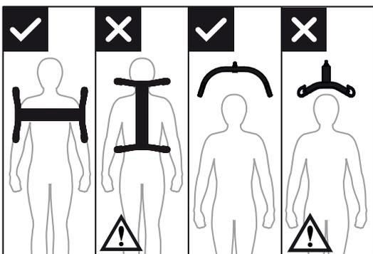
The suspension must always be positioned across the user, to prevent the user from unintentionally sliding out of the sling.
