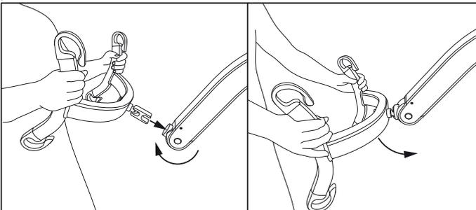
Insert bolt on suspension in connection point to mount suspension. When bolt is completely inside the suspension is mounted and can rotate freely.
