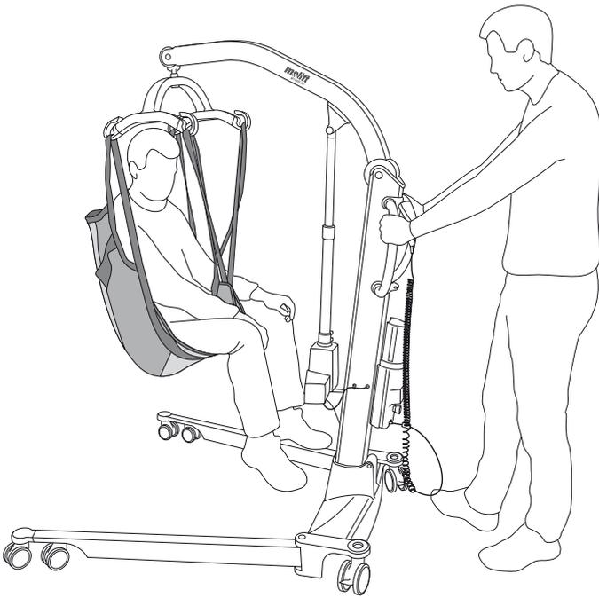
Try to position the user as low as possible (preferably resting the feet on the chassis) when transferring the lifter with a suspended user. In this way the centre of gravity will be low and reduce the risk of instability.
