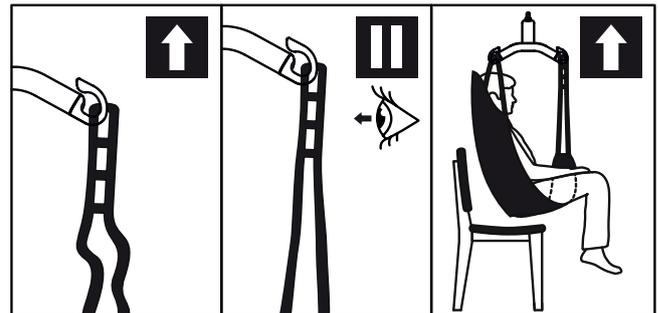
1. Check that the sling is correctly fitted around the user and that the strap loops are correctly fitted to the suspension hooks.
