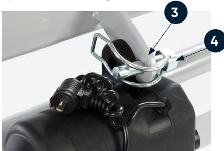
2 | Pin removed and holes aligned.
