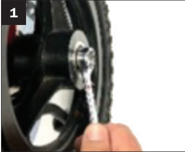
1. Loosen wheel with 5/8” wrench.
