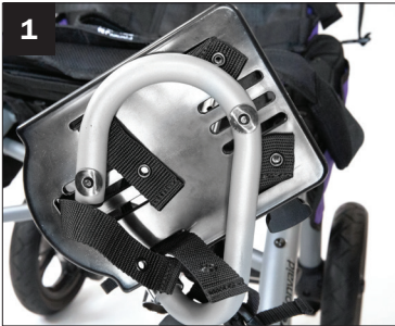
1. To attach foot positioner, thread strap through footplate.
