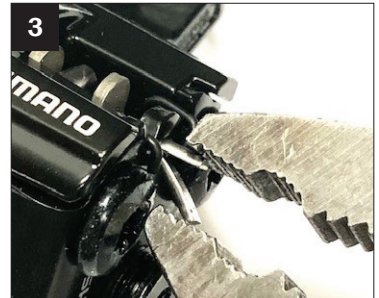
3. Remove cotter pin with pliers.
