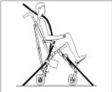
Correct positions of shoulder and lap belt restraints and wheelchair tiedowns.
