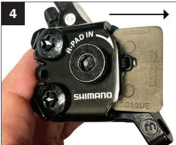
4. To remove pads, push pads through caliper.
